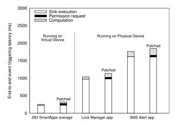
Fig. 5: Breakdown of the end-to-end event trigger latency with and without ContexIoT patching on virtual and physical devices
